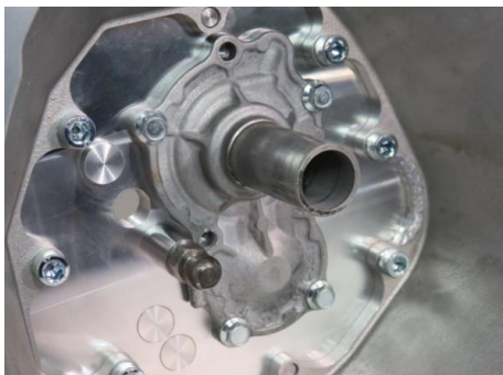
⑤ Temporary installation of front cover
