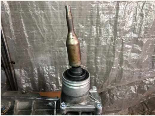
Neutral position before replacement (housing inverted 180° )
