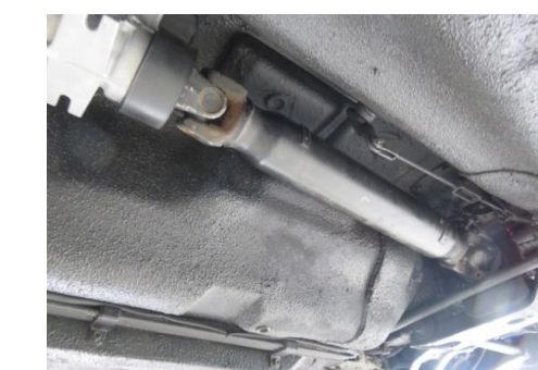
Example of S30 shaft installation without machining
