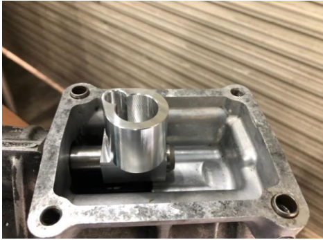
① Shift Striking installed
